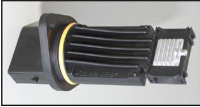
**Air mass flow sensors such as the PB-LMS by EngineSens work on the principle of the hot-film anemometer. The manufacturer said that they are often used in cogeneration plants to monitor the soot in the exhaust gas duct in the area before the heat exchangers.**
